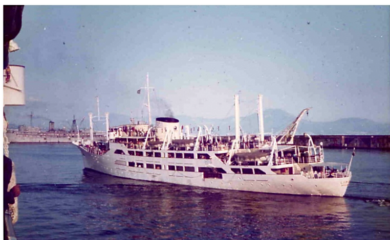
The motor vessel Lipari (dimensions: 86.63 metres by 11.55 metres). Net tonnage 884.98 tonnes.
