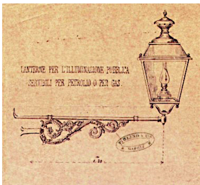
The type of lamp used in Naples, convertible from vegetable gas to fossil gas.
