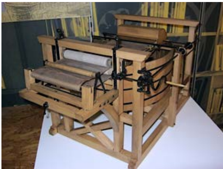
Prototype of the first Continuous or Endless Machine (Sans Fin) by Louis-Nicolas Robert.
