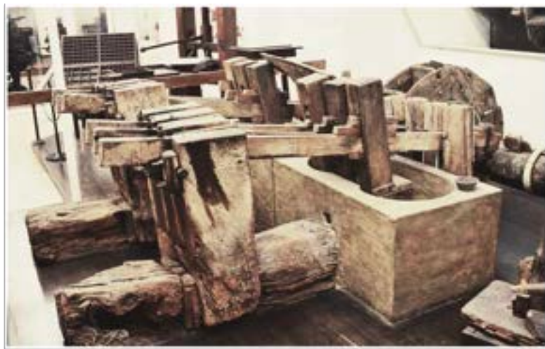
Antique hydraulic pile with multiple hammers. Fabriano Paper Museum.
