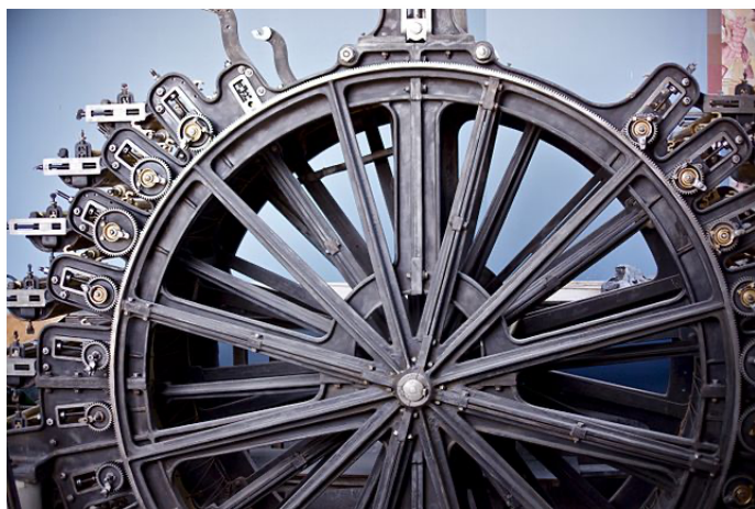
Isidore Leroy's 26-colour machine was based on the Potter & Ross model.
